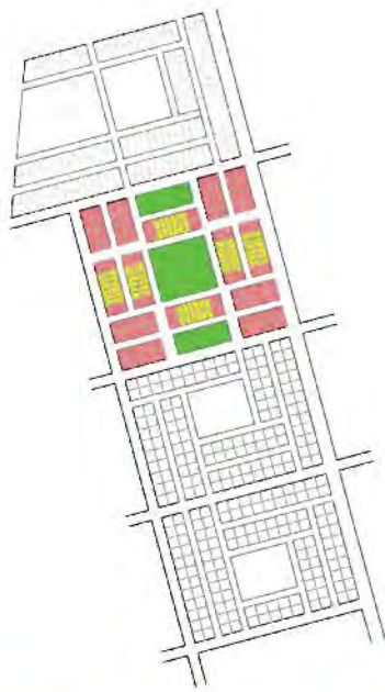
FIG 20. MODIFIED BUILDING BLOCK Redesign building blocks by mixing plot sizes, and providing for public space along the roads.
