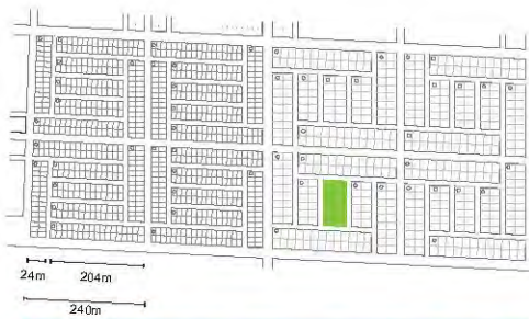
FIG 14. CURRENT BUILDING BLOCK KALAY Segregated plot sizes, very large blocks and very little public space.
