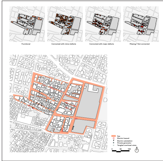
Graphic 6: Map of a neighbourhood electrical network. Source: UN-Habitat and UNICEF Neighbourhood Profiling in Lebanon
