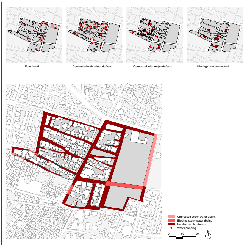
Graphic 9: Mapping a neighbourhood storm water network. Source: UN-Habitat and UNICEF Neighbourhood Profiling Project in Lebanon
