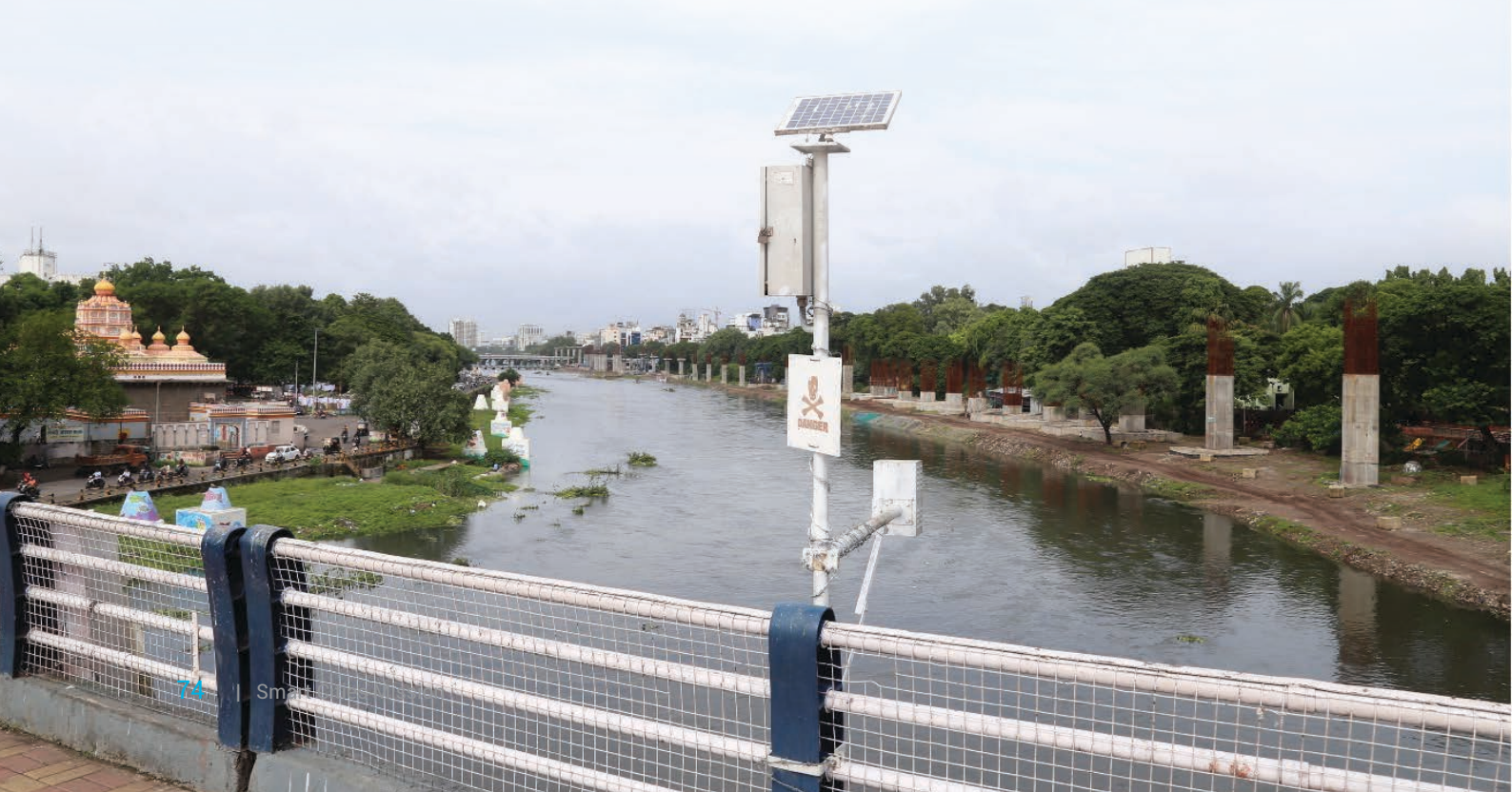
Image 33: Pune Smart City has installed more than 50 flood sensors at strategic locations as part of an integrated approach to disaster risk management. Source: Pune Smart City
