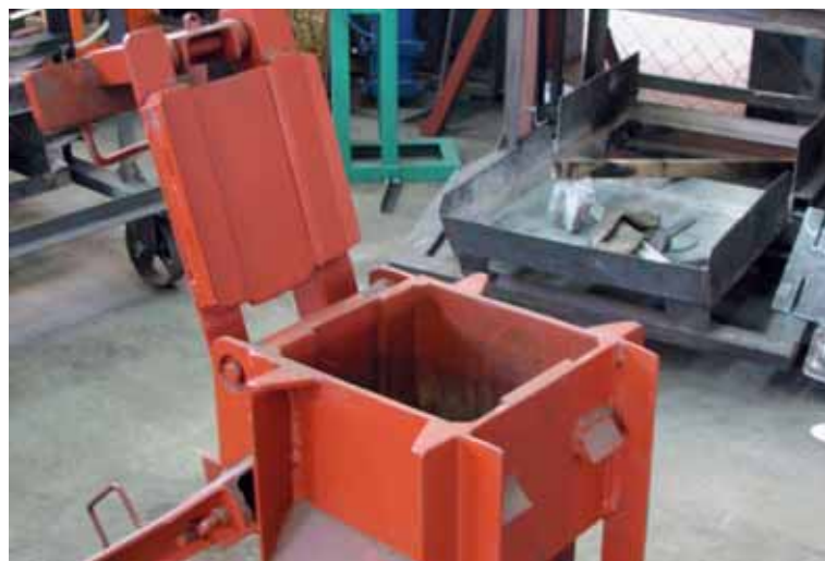
Figure 80. TDAU hand press for Hydraform blocks. Photo © UN-Habitat
